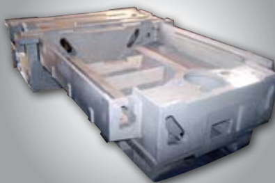
Machining centre base iron castings, EN-GJL-300
